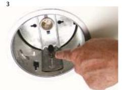
Deep set the light socket by loosening the wing nut. Push down the socket and tighten the nut. Adjust as needed. Bulb should almost be touching baffle for best look. It may take several attempts.
