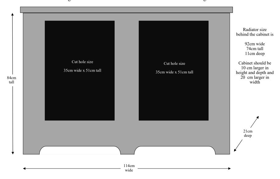
Beaux-Artes decorative HVAC grilles can also be used with radiators. They must be integrated with a custom made box as shown above. This design features two of our RR-209 20x14 Louis XIV style grilles. In this case the grilles are mounted to the front surface of a MDF radiator cover. Radiators should be spray painted with flat black paint so that they disappear behind the grilles. .....stuart@beaux-artsclassicproducts.com
