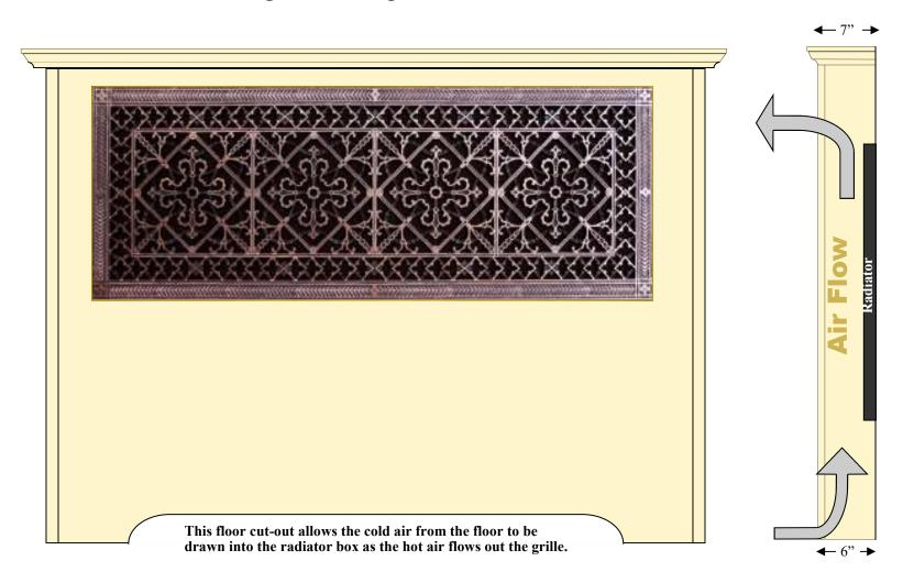
Beaux-Artes decorative HVAC grilles can also be used with radiators. They must be integrated with a custom made box as shown above. This design features our RR-209 12x36 Arts & Crafts style grille. The grille should be mounted no closer than 4" from the front surface of the radiator. In this case the grilles are mounted to the front surface of the wooden radiator cover. Radiators should be spray painted with flat black paint so that they disappear behind the grilles.
