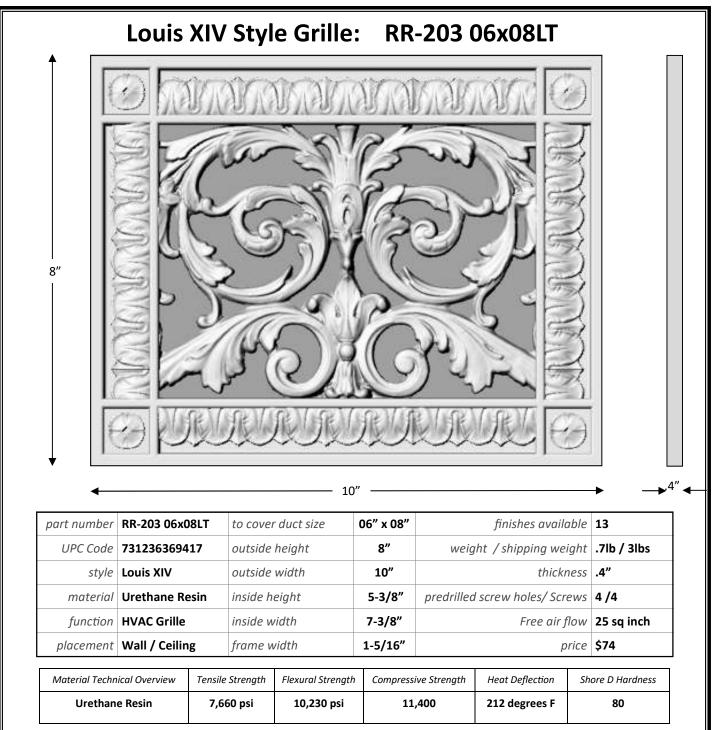
Beaux-Arts Classic Products' grilles are designed for wall and ceiling use only, and not suitable for floor use. They are virtually maintenance free, cast from an exterior grade urethane resin. They are also quiet, since resin doesn't vibrate. In addition resin won't rot, rust, corrode or grow mold.
