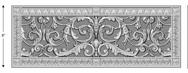
part number RR-203 06x20LT to cover duct size 06" x 20" finishes available | 13 **UPC** Code outside height 8" weight / shipping weight | 2lbs / 7lbs style Louis XIV 22" outside width thickness material Urethane Resin inside height 5-3/8" predrilled screw holes/ Screws 6/6 function | HVAC Grille 19-3/8" inside width Free air flow 65.6 sq inch placement | Wall / Ceiling frame width 1-5/16" price \$119
