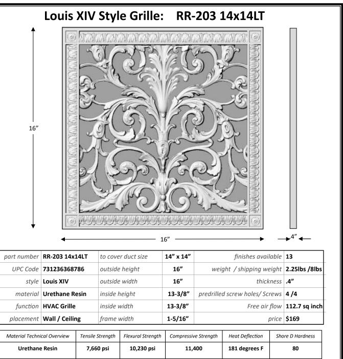
Beaux-Arts Classic Products' grilles are designed for wall and ceiling use only, and not suitable for floor use. They are virtually maintenance free, cast from an exterior grade urethane resin. They are also quiet, since resin doesn't vibrate. In addition resin won't rot, rust, corrode or grow mold.
