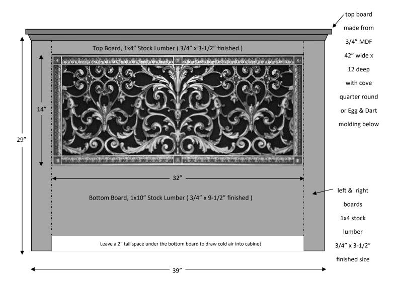
The cabinet can be made from pre-painted stock lumber purchased from Home Depot or Lowes. It will look best if the grille is installed sunken into the surrounding stock lumber, rather than on top of the stock boards. 1/2" plywood strips can be used on the back of the stock lumber front to allow the grille to be installed sunken into the surrounding stock lumber.
