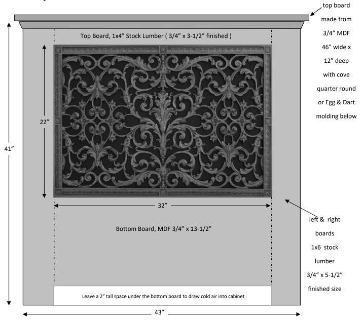
The cabinet can be made from pre-painted stock lumber purchased from Home Depot or Lowes. It will look best if the grille is installed sunken into the surrounding stock lumber, rather than on top of the stock boards. 1/2" plywood strips can be used on the back of the stock lumber front to allow the grille to be installed sunken into the surrounding stock lumber
