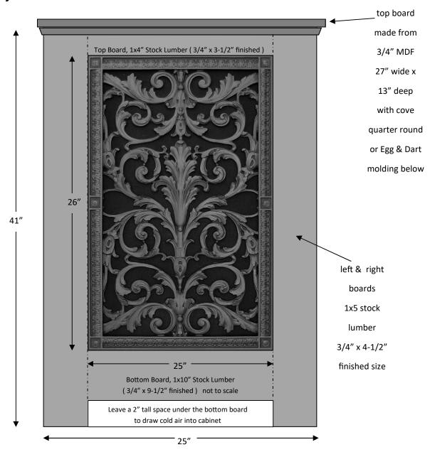
The cabinet can be made from pre-painted stock lumber purchased from Home Depot or Lowes. It will look best if the grille is installed sunken into the surrounding stock lumber, rather than on top of the stock boards. 1/2" plywood strips can be used on the back of the stock lumber front to allow the grille to be installed sunken into the surrounding stock lumber.
