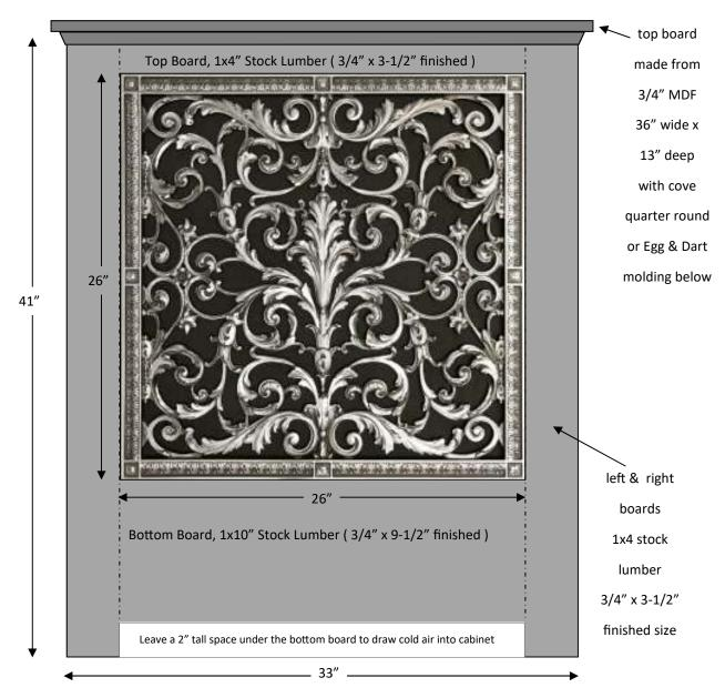
The cabinet can be made from pre-painted stock lumber purchased from Home Depot or Lowes. It will look best if the grille is installed sunken into the surrounding stock lumber, rather than on top of the stock boards. 1/2" plywood strips can be used on the back of the stock lumber front to allow the grille to be installed sunken into the surrounding stock lumber.
