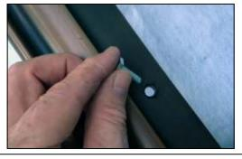
Insert the two 3/4" bolts into the two countersunk holes on the front of Base-Frame.
