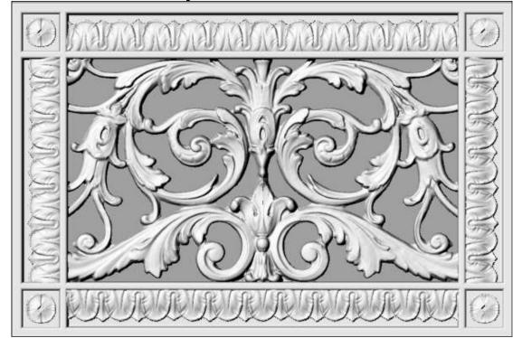
06" x 10" RR-203 06x10LT finishes available | 13 part number to cover duct size 8" UPC Code | **731236369455** weight / shipping weight | .8lb / 3lbs outside height style Louis XIV outside width 12" thickness 3/8" 5-3/8" material Urethane Resin inside height predrilled screw holes/ Screws 4/4 function HVAC Grille inside width 9-3/8" Free air flow 31.7 sq inch
