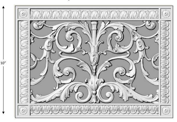
part number | RR-203 08x12LT 08" x 12" to cover duct size finishes available **13** weight / shipping weight | 1.25lb / 5lbs *UPC Code* **731236368403** outside height 10" 14" thickness 3/8" style Louis XIV outside width 7-3/8" predrilled screw holes/ Screws 4/4 material Urethane Resin inside height 11-3/8" Free air flow 52.9 sq inch function | HVAC Grille inside width placement | Wall / Ceiling frame width 1-5/16"
